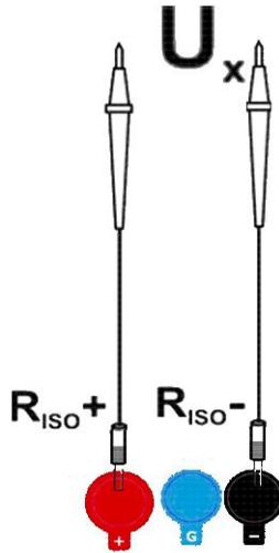
Connect the meter to a voltage source.
