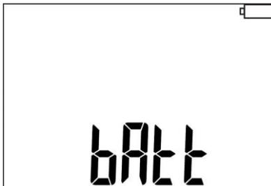
The battery pack is fully discharged, all measurements are blocked. The meter switches off automatically after 5 sec.
