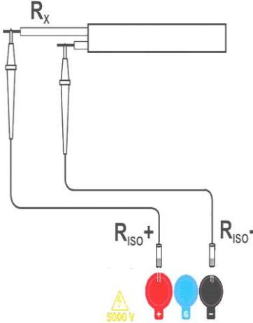
Connect test leads according to the drawing.
