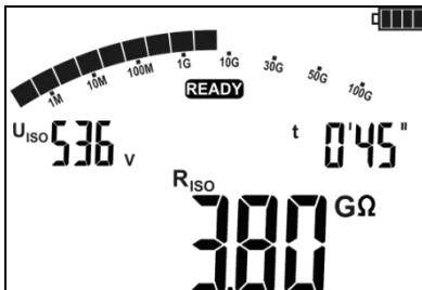
After the measurement is completed or stopped, read the result. The results of all completed measurements will be displayed (even when the measurement was interrupted) When the meter switched into standby mode, the measurement result may be recalled by pressing **ENTER**.
