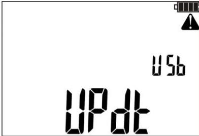
2. Connect the cable to the USB port of the computer and the USB socket of the meter.
