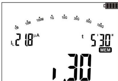
The value of leakage current  $I_L$  measured in time  $t=5'30''$ . Symbol  $i_{30}$  indicates the selected time interval, in which the leakage current value was recorded.
