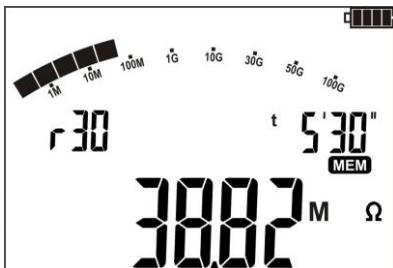
Resistance  $R_{ISO}$  value, measured in time  $t=5'30''$ . Symbol  $r_{30}$  indicates the selected time interval, in which the resistance value was recorded.
