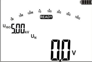
The meter indicates readiness for measurement with increasing voltage.
