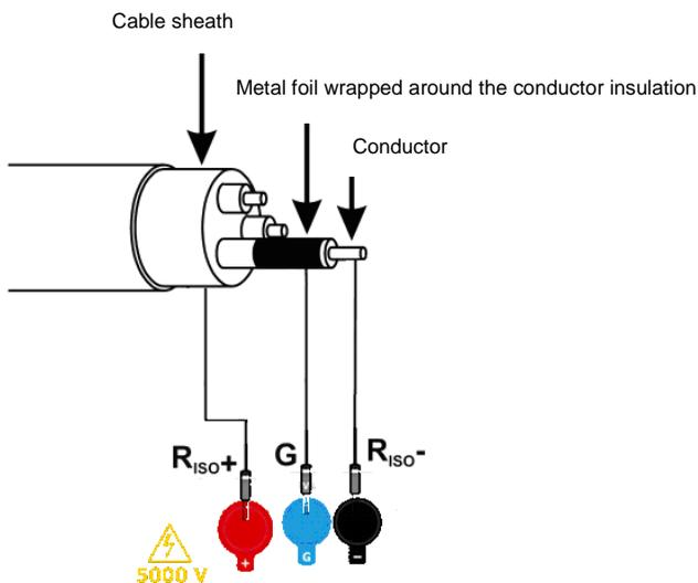
The same shall apply when measuring the resistance between two conductors of the cable, attaching to **G** terminal other conductors that do not take part in the measurement.
