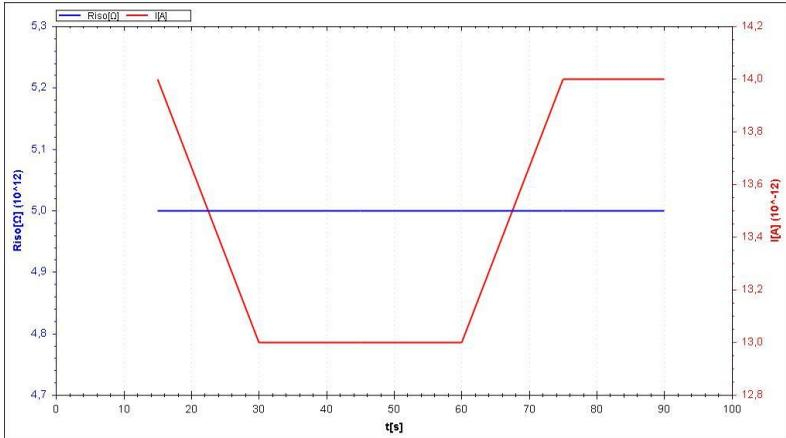
For a measurement with voltage increase method (RampTest), the user basing on performed measurements, may analyse the characteristics of voltage, resistance and current as a function of time.
