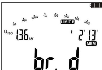
If the electric resistance strength of the tested insulation is exceeded and the puncture occurs, the main field of the display will show message **br. d** - breakdown.
